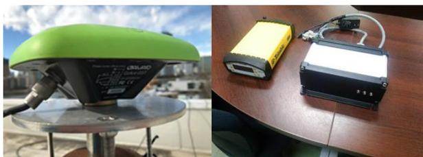
Fig. 21. Antenna (GrAnt-G5T) and Receivers (SPS855 and Magellan)
