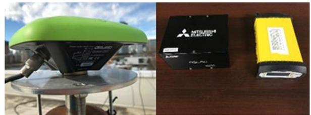
Fig. 7. Antenna (GrAnt-G5T) and Receivers (AQLOC and SPS855)
